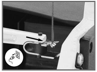
Figure 3. V-notch on lower blade holder.
